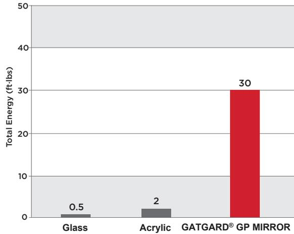
\*Instrumented Impact per ASTM D3763, sample thickness is 0.118" nominal
