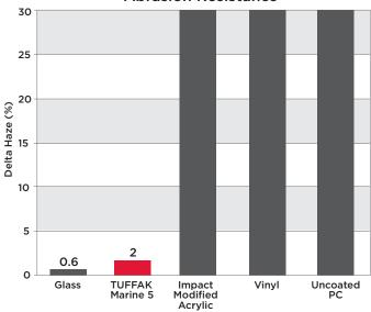
\*Taber Abrasion per ASTM D 1044, 100 cycles, CS-10F wheels at 500 g load
